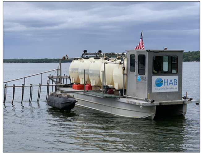
The HAB Aquatic Solutions barge injects alum into East Balsam Lake.
