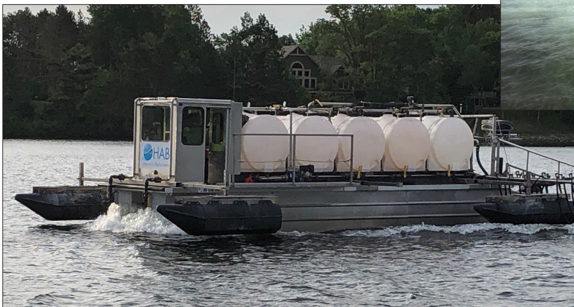
Left: The HAB Aquatic Solutions barge applies aluminum sulfate in our first East Balsam alum treatment on June 14, 2020. Above: The "floc" visible in the water.
