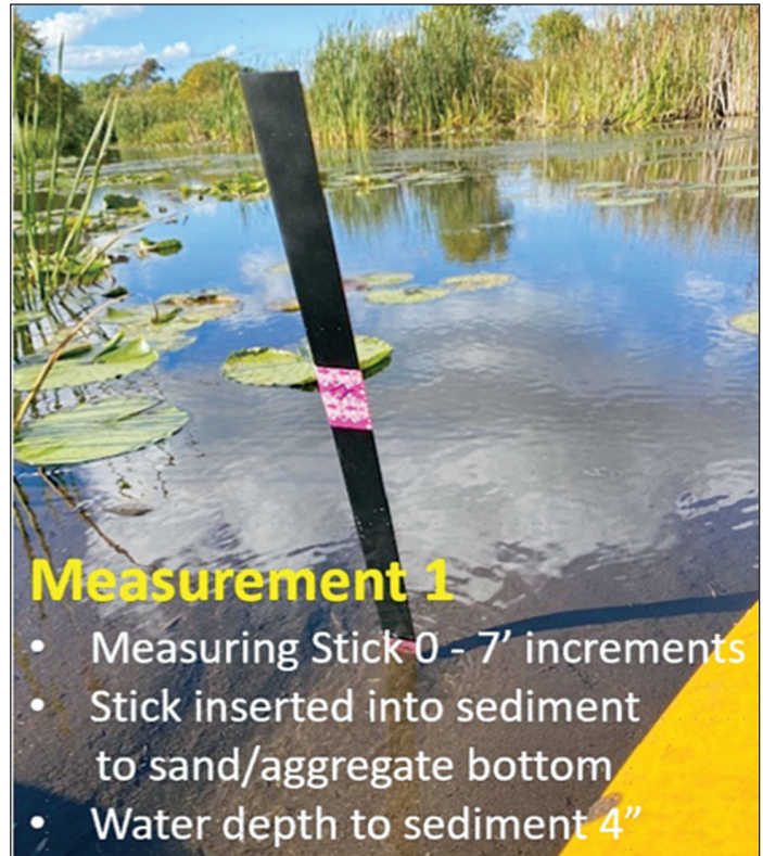
Measurements of the sediment levels were taken where Rice Creek enters the sedimentation pond. The water depth to sediment is four inches in the measurement area outlined in yellow, above.
