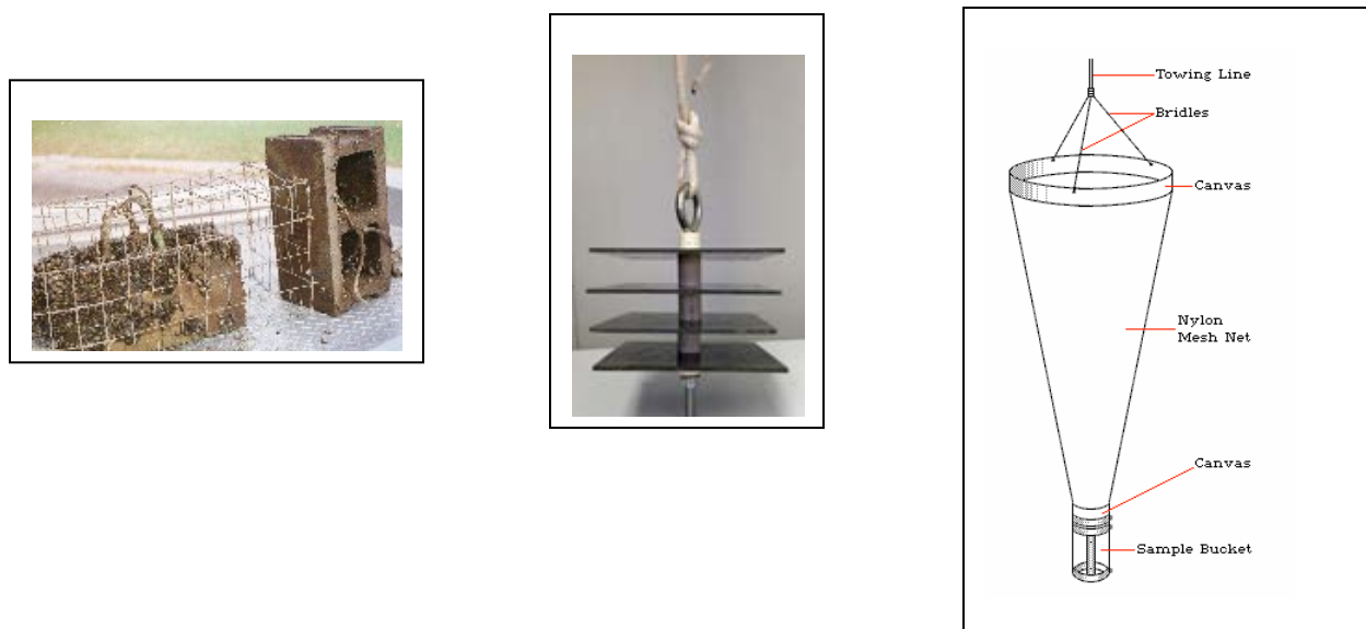
Figure 23. Monitoring Equipment: Cinder Blocks, Sampling Plates, and Nets for Veliger Tows
