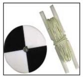
Figure 0: Secchi Disk is a 7" round disc used to measure water clarity.
