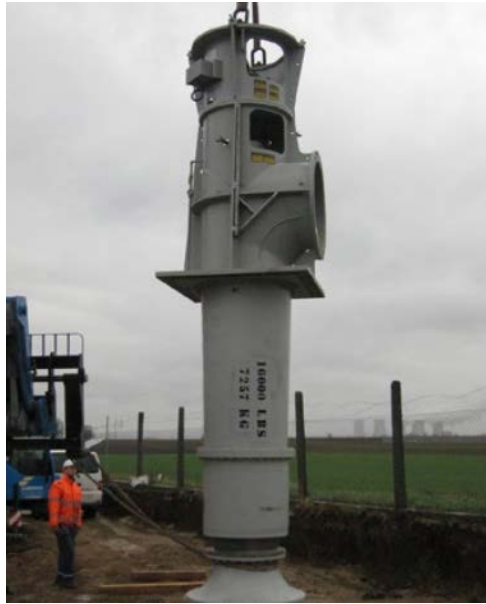
Figure 5-5: 430 cfs Pump, Flygt A-C Series Column Pump (Flygt 2014)
