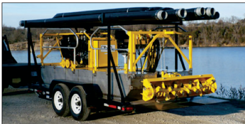
Small and transportable dredging unit
