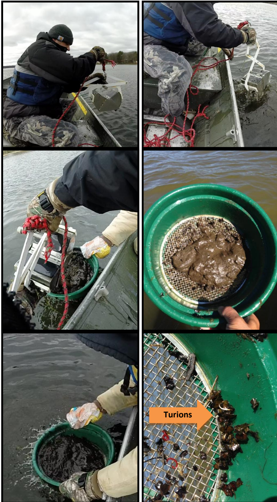
Figure 4: East Balsam Ponar Grab and Turion Sieving
