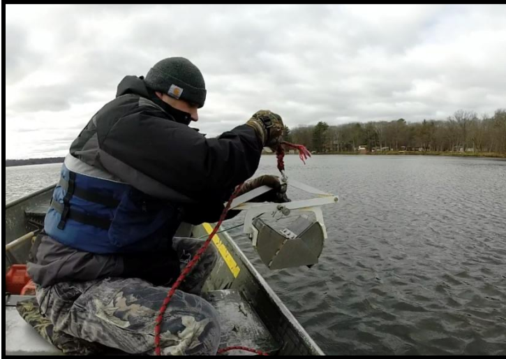
B. Collins Lowering the Ponar Dredge – East Balsam
